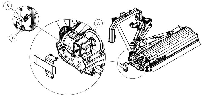
Recommended oil: Gearbox oil Mereta 150 or Mereta 220 synthetic oil (Statoil) or Esso Syntetic EP150.
